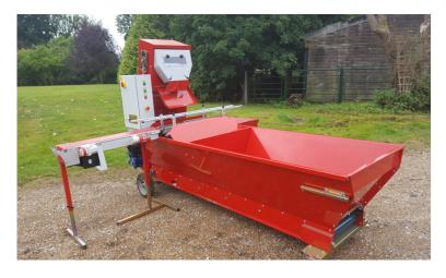
The G100 Pot topper is a fast and accurate filling system for the topping and settling pots from 1ltr to 10ltr.
